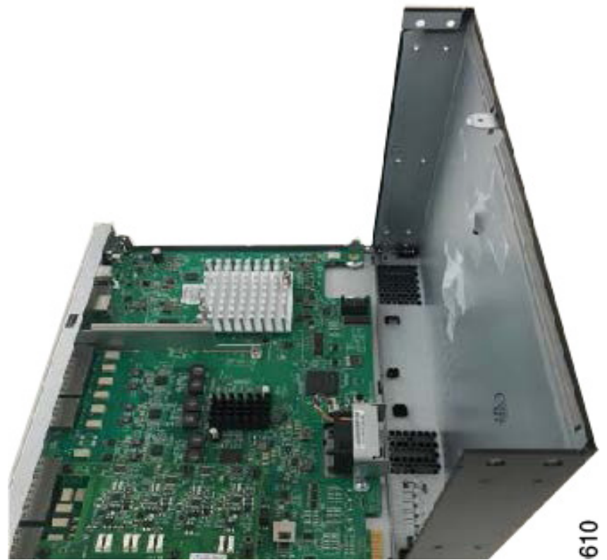
Figure 5-55 Cisco 4321 ISR Chassis Cover
