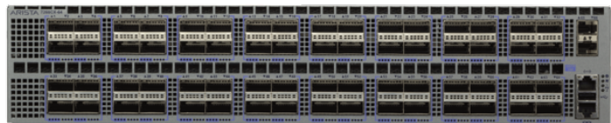
Arista 7260CX-64: 64 x 40/100GbE QSFP100ports, 2 SFP+ ports
