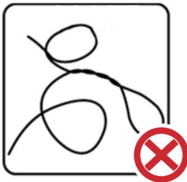
Figure 3-45 Circled or twisted cables
