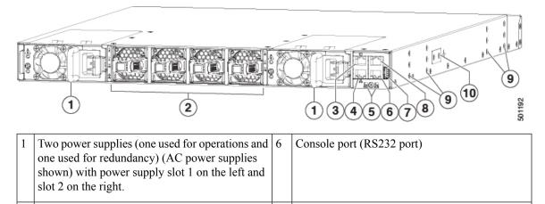
Four fan modules with fan slot 1 on the left and
